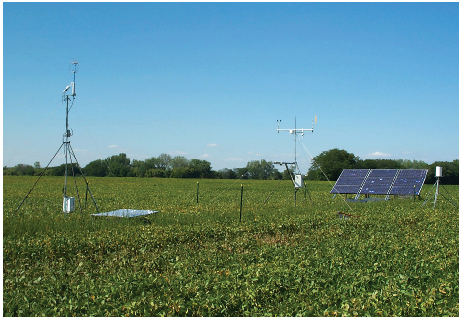
A solar-powered eddy flux tower located at a soybean field at Fermilab is measuring the exchange of carbon dioxide between plants and soil and the atmosphere to study the carbon balance of agricultural fields typical of the U.S. Midwest.
