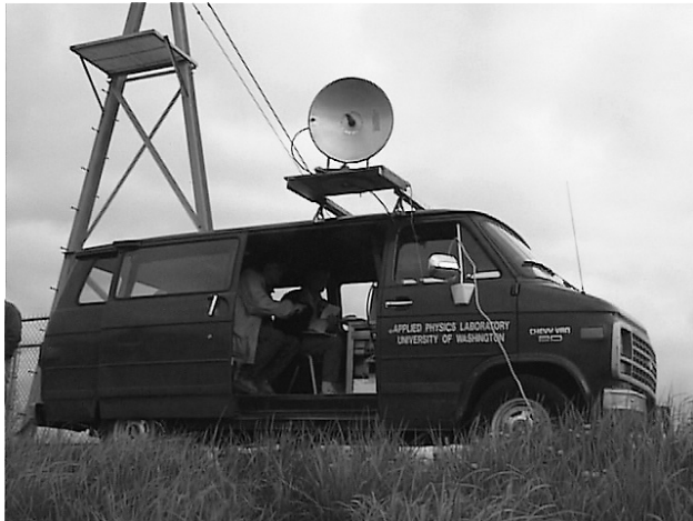
Figure 4. Van-mounted side-looking back-scattering microwave (gigahertz) radar system for acquiring surface-velocity data (after Costa and others, 2000).
