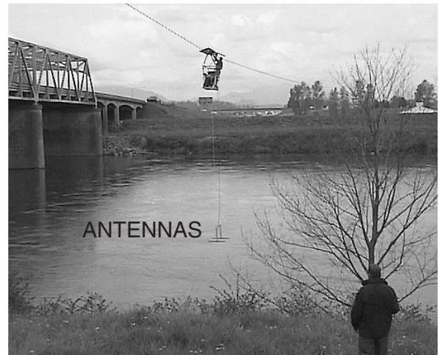
Figure 1. Ground-penetrating radar system mounted inside cableway car with 100 mega-hertz antennas suspended 0.5 to 3 m above the water surface.
