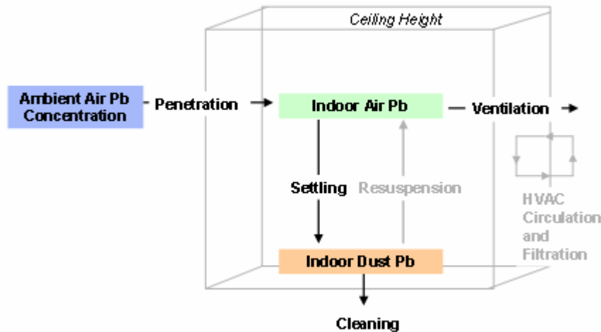
Exhibit G-3. Mechanistic Indoor Dust Model Schematic
