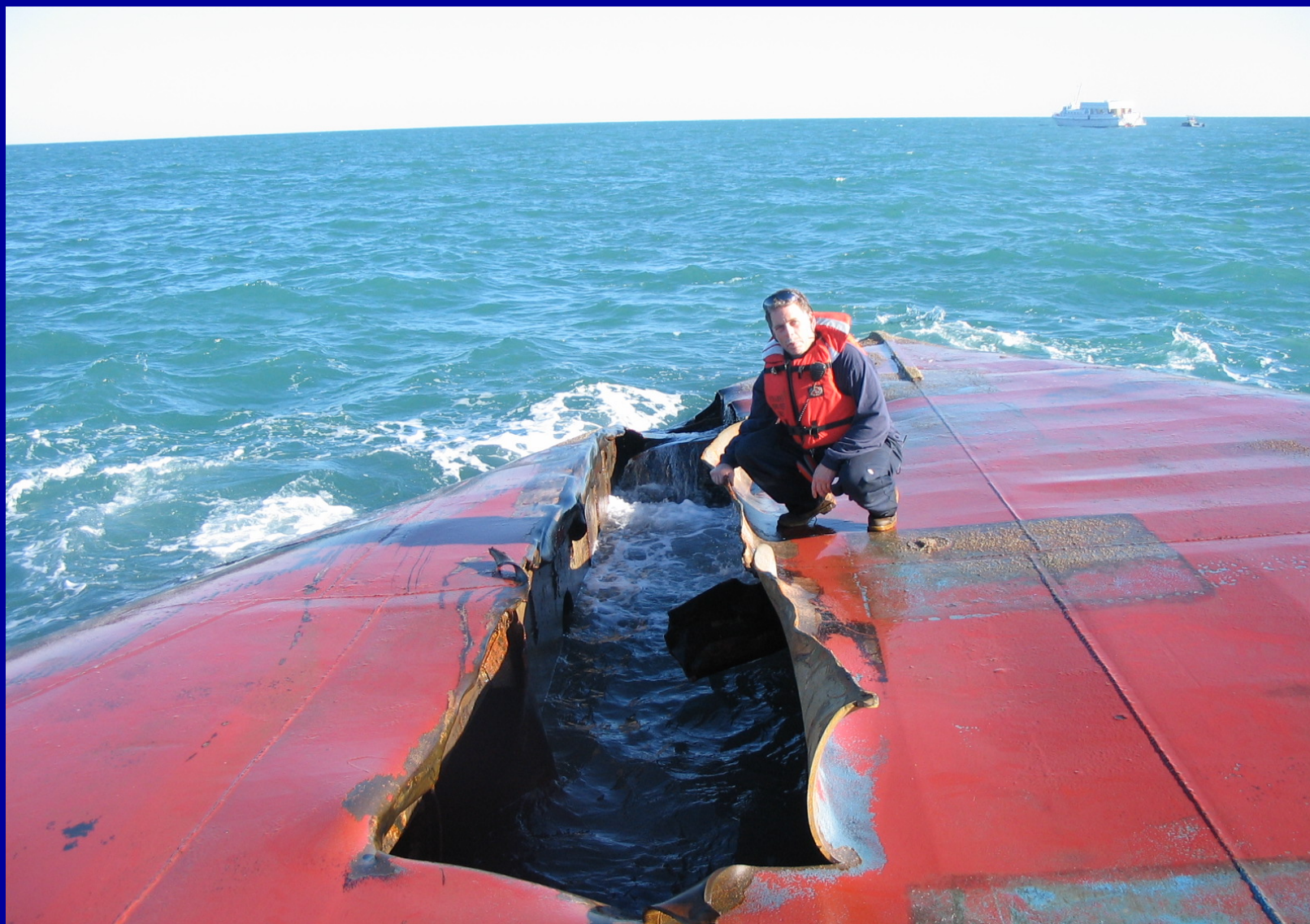
A large gash in the hull of the now completely inverted DBL 152.
