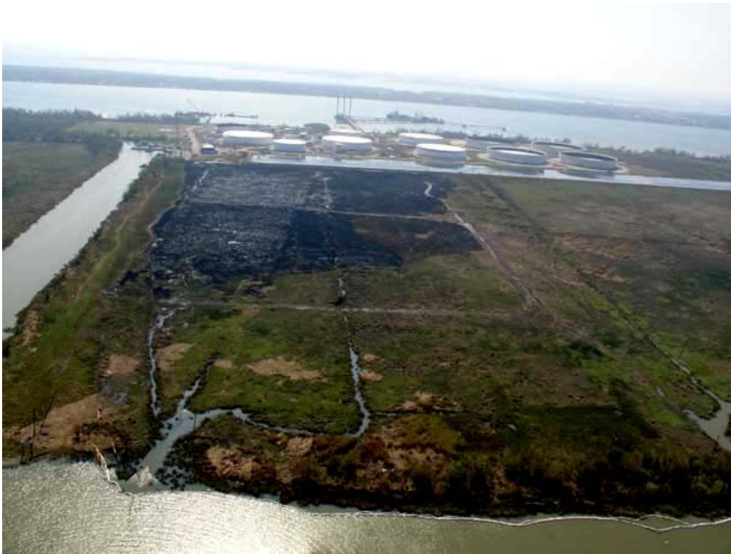
Figure 16. Final Footprint of the burn area. Note Zone 2 is about 85% burned, but Zone 5 only about 50% is burned.
