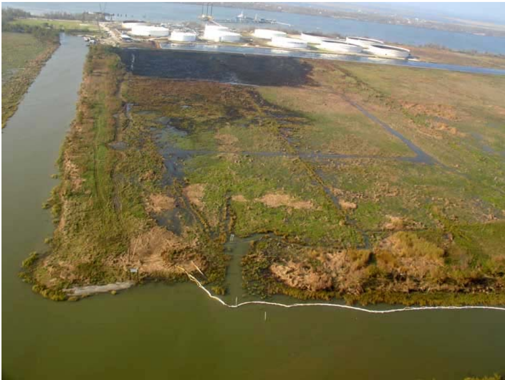
Figure 11. Post-Burn Day 1 (October 12, 2005). All zones are clearly visible. Burned Zones: 1 and 4. Oil contamination visible in Zones 2 and 5. Zones 3 and 6 are in the fore front.
