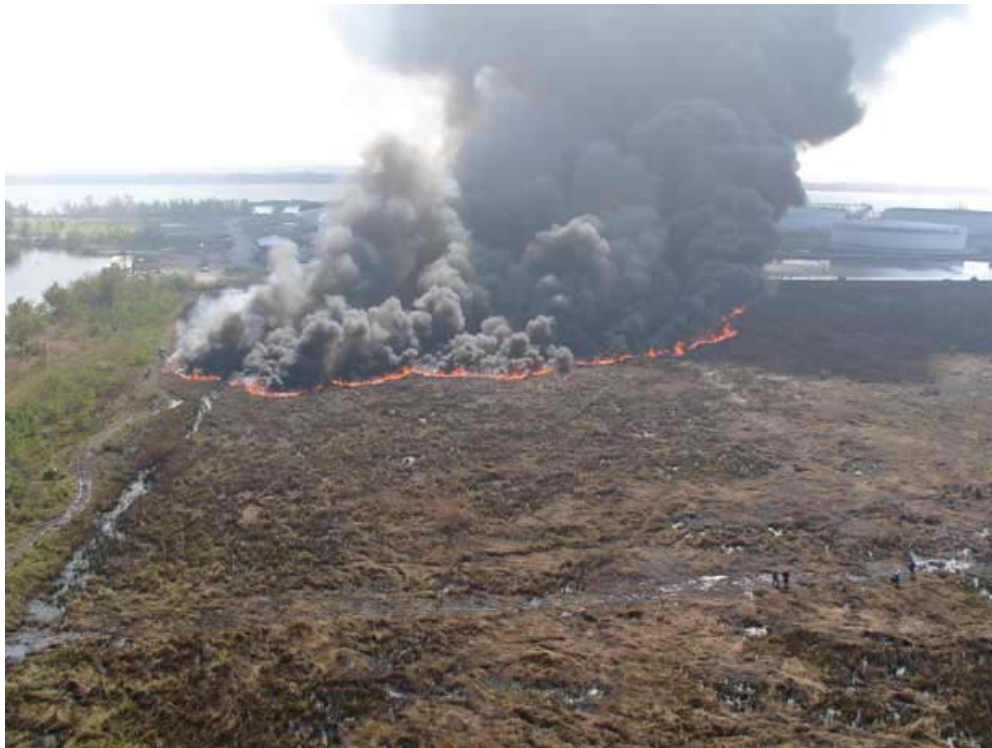
Figure 7. Aerial photo 1.25 hours into the burn (October 12, 2005). The fire has burned about a third of Zone 1, and has crossed the boundary into Zone 4. The people standing in the bottom right hand corner of the photo are behind the fire breaks of Zone 1.
