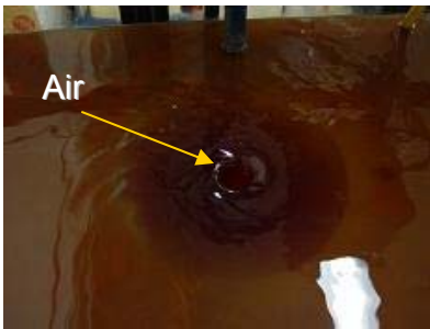
Air starts to enter the pump (c)
