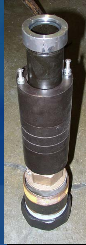
Overfill protection valve
