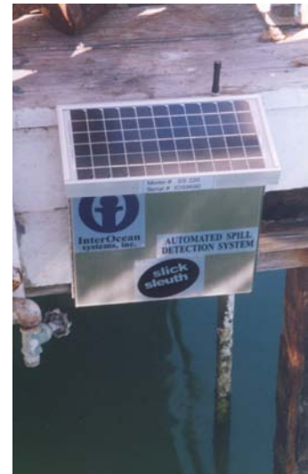
Figure 4. Early production unit. DC/Solar power, radio
