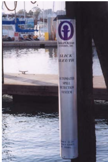
Figure 3. Prototype spill sensor. Installed near fuel pier (background).
