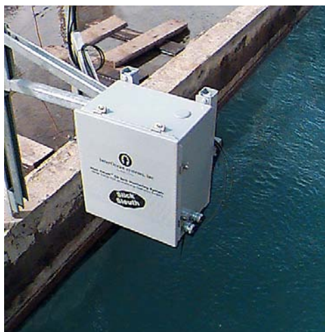
Figure 6. One of 5 units deployed at a Shell refinery (Australia) to monitor cooling water outfall channels. Photo courtesy Shell.
