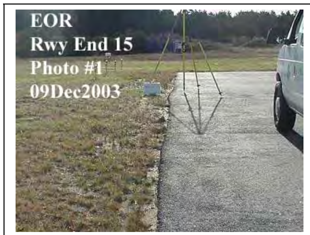
Figure-3-3: Photograph Type #1 (Eye Level). Photo taken from above the mark, showing an area around the mark about 1 meter in diameter.
