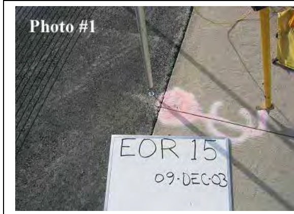
Figure-3-3: Photograph Type #1 (Eye Level). Photo taken from above the mark, showing an area around the mark about 1 meter in diameter.
