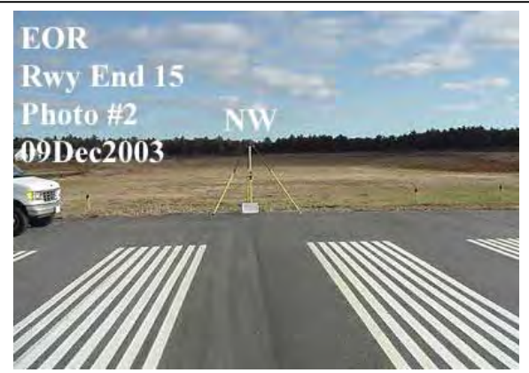
Figure 3-4: Photograph Type #2 (Approach). Photo showing tripod over the mark in foreground and approach in the background.
