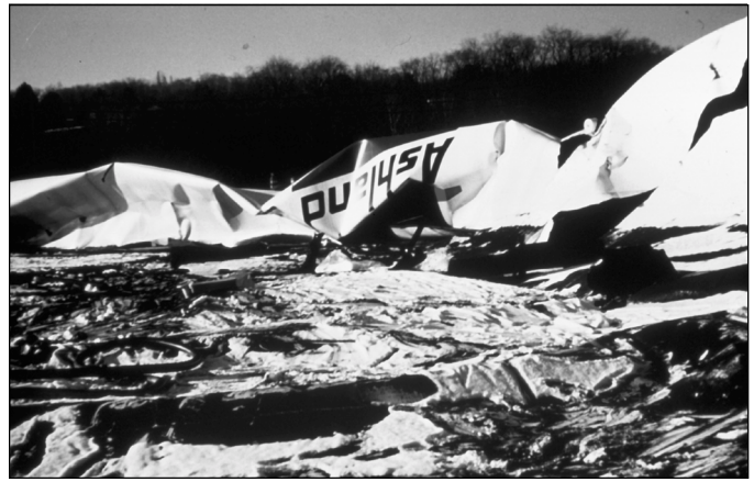
The Ashland storage tank split when filled to capacity.
