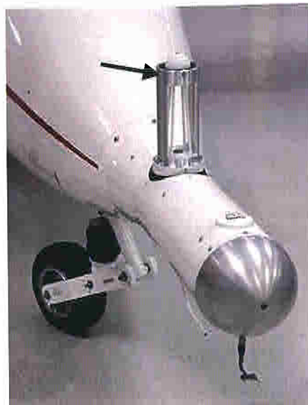
Figure 2. Stiffened Licor Mount
