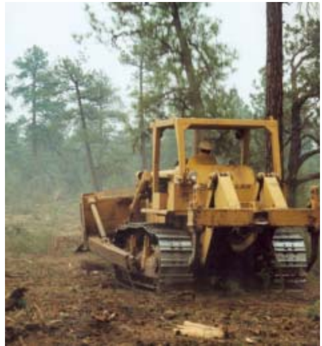
A bulldozer operator knocks down trees to create a safety zone for firefighters and fire equipment south of Show Low, AZ. Photo by Tom Schafer.
