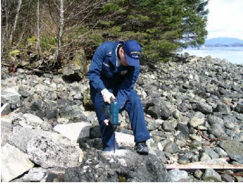
Ensign Matthew Glazewski of NOAA Ship FAIRWEATHER drills to establish a benchmark on Noyes Island, AK.
