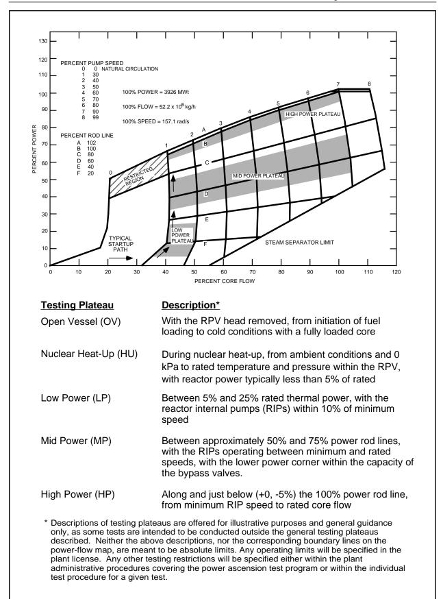
Figure 14.2-1 Power-Flow Operating Map and Testing Plateau Definitions
