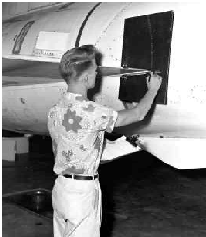
NASA Photo E-1005. Flap Calibration
