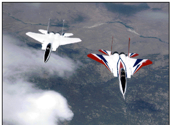
NASA Dryden's two F-15B aircraft fly in tight formation during a research mission. The F-15 ACTIVE, right, is distinguished by the canards mounted outside the engine air inlets and by its distinctive red, white, and blue color scheme. NASA photo EC96 43656-1
