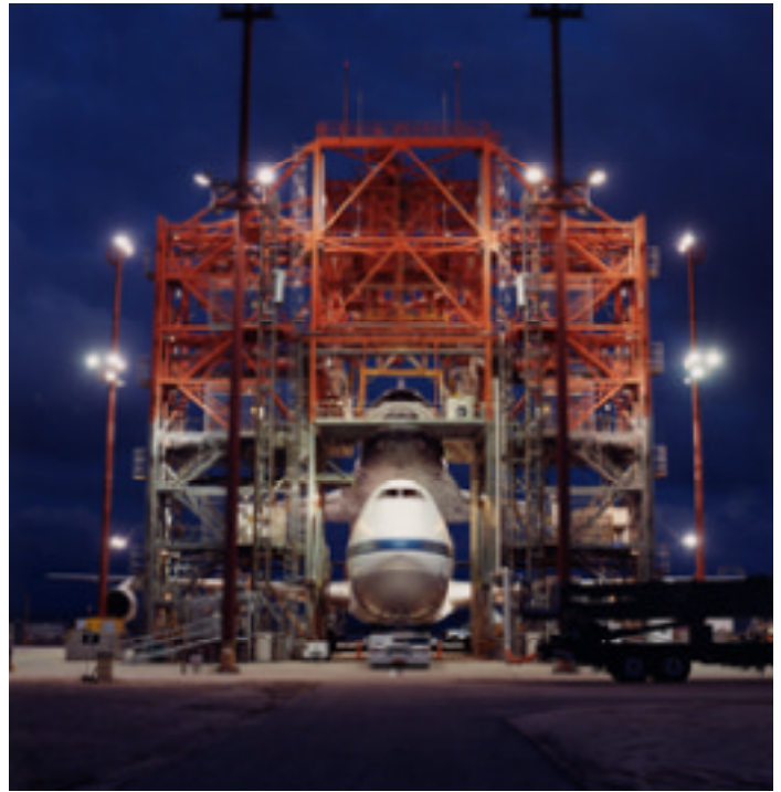
EC01 0041-15 The Space Shuttle Atlantis is placed atop Shuttle Carrier Aircraft 911 while inside the MDD in preparation for its March 1, 2001, departure to the Kennedy Space Center.
