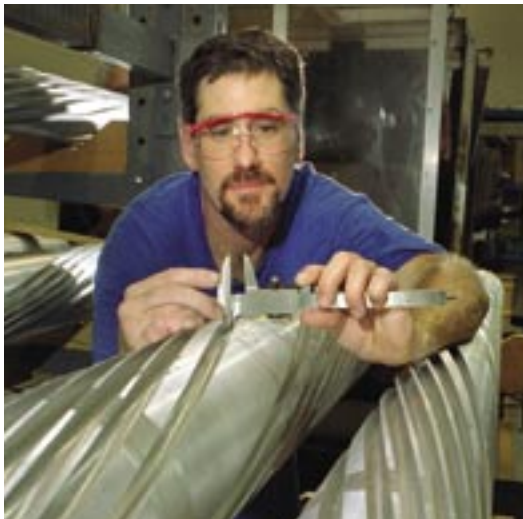
Special magnets with a corkscrew-like design, known as Siberian Snakes, regularly flip the spins of protons during RHIC spin experiments to keep the protons in the beam aligned, or polarized.
