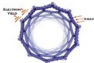
A front view of a carbon nanotube. During NEXAFS analysis, x-rays are directed at the nanotube and are absorbed by some of its electrons.
