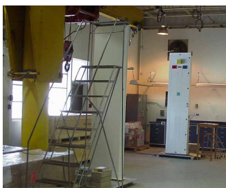
A portal radiation detector is set up for testing in Brookhaven's indoor assembly and evaluation facility.
