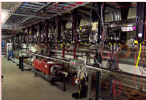
The MI tunnel near MI-31. Top (inside black support structure): Recycler beam line with cooling tanks. Middle (above red magnet): return line for electrons. Bottom: MI beam line with magnet (red), with parts of the beam pipe removed. (Click on image for larger version.)
