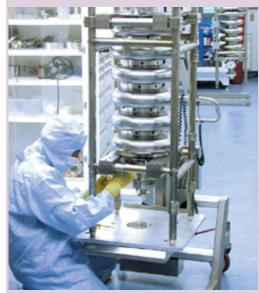
A superconducting RF cavity for the Spallation Neutron Source is assembled in a clean room of the Test Lab at Thomas Jefferson National Accelerator Facility. (Click on image for larger version.)
