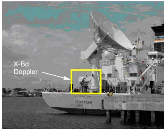
Continuous Pulse Doppler X-Band Radar 1.6 KW peak transmit power 0.14 M/S Doppler velocity resolution 4 x 4 M reflector size
