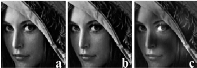
FIG. 1. Image reconstruction of oversampled diffraction patterns as a function of the number of missing waves. (a) \eta_x, \eta_y = 1 . (b) \eta_x, \eta_y = 2 . (c) \eta_x, \eta_y = 4 .
