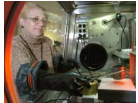
R&D 100-award winner Jacqueline Johnson prepares a small sample of a ceramic glass that formed the basis for radiographic imaging plates that she and her colleagues developed in order to allow doctors to obtain clearer, more-detailed mammograms.
