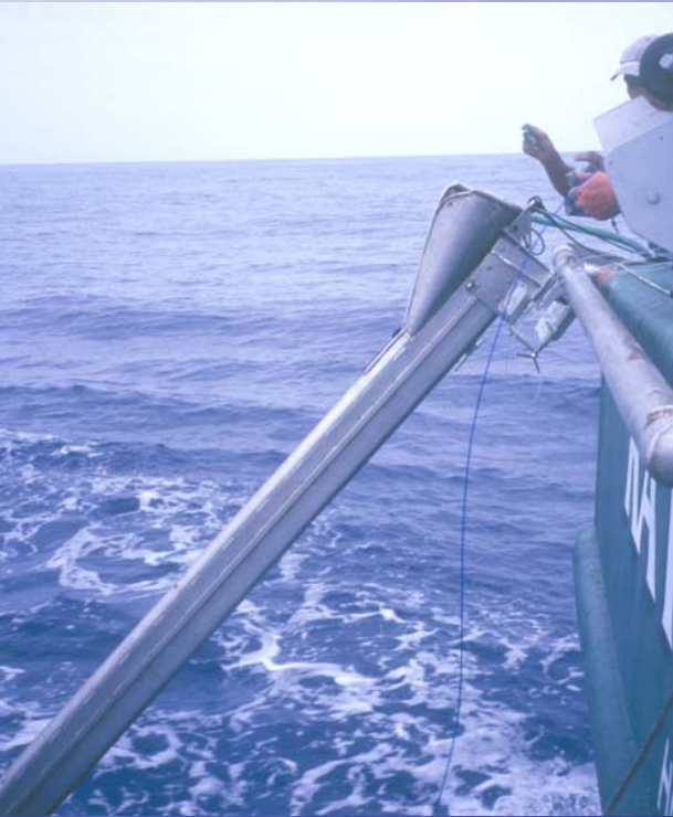
Underwater setting chute
