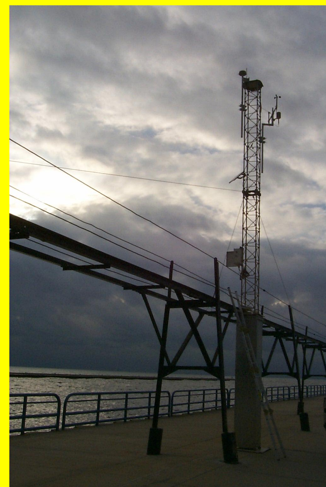
Figure 8. Meteorological station on the St. Joseph pier. Similar sites have been installed at Michigan City and Kenosha, Wisconsin.
