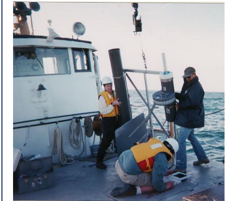
Eleven of these sequential sediment samplers developed at GLERL were deployed in southern Lake Michigan to collect plume particles as they settle towards the lake bottom. The traps are programmed to collect 23 samples over a period of 10 days each.
