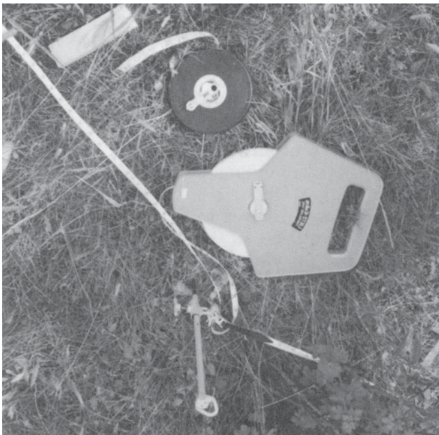
Figure 18. Two common measuring tapes.
