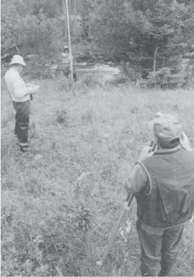
Figure 49. Good location for level setup.
