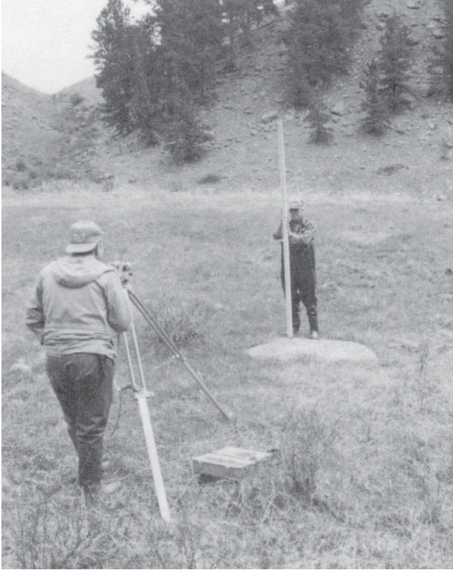
Figure 34. Shooting the elevation of the benchmark.
