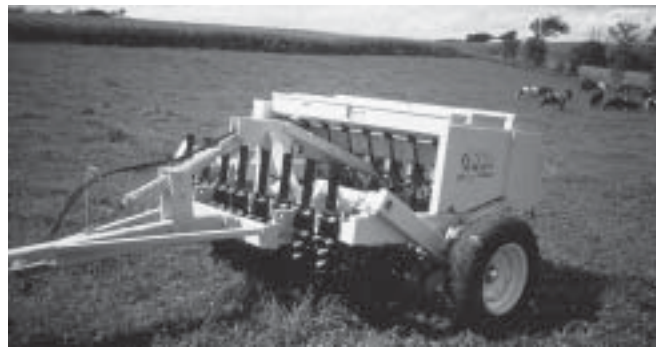
Figure 15 —Truax drill with three seed boxes and three sets of drops that can seed three different seed mixes or species at the same time at different rates and depths.
