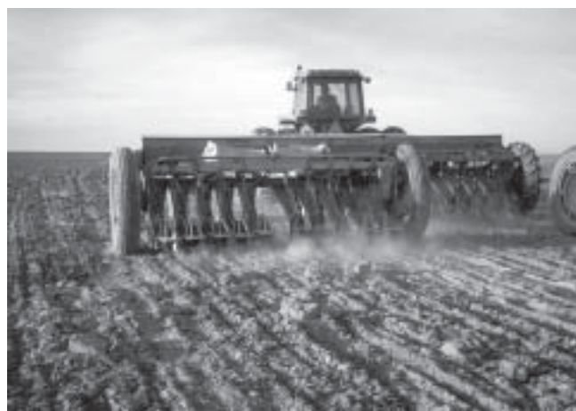
Figure 13 —Three Rangeland drills with drag pipes and depth bands.
