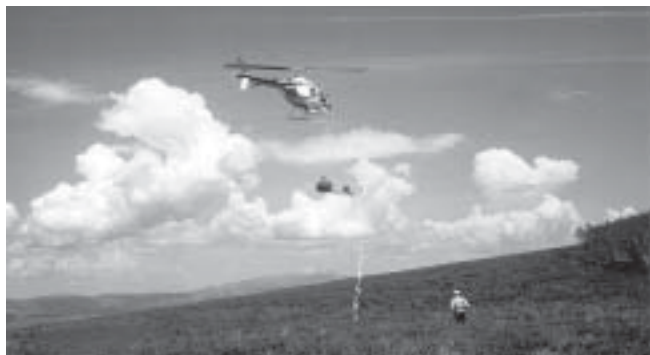
Figure 37 —Helitorch used to start a prescribed burn in a mountain big sagebrush community.
