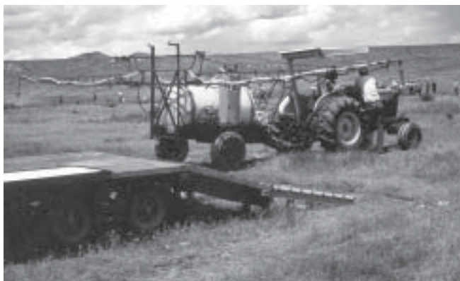
Figure 39 —Rangeland boom sprayer. Booms must be mounted high enough to clear tall shrubs.
