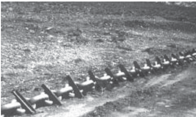
Figure 6—Ely chain. Anchor chain with railroad rails welded crossways on every other link.
