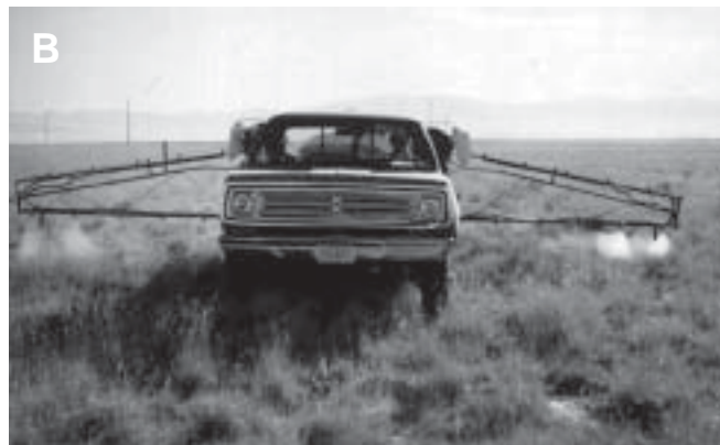
Figure 4 —Boom sprayers can be (A) hand held and (B) vehicle mounted. Spraying strips of crested wheatgrass with Roundup to facilitate transplanting desired shrubs.
