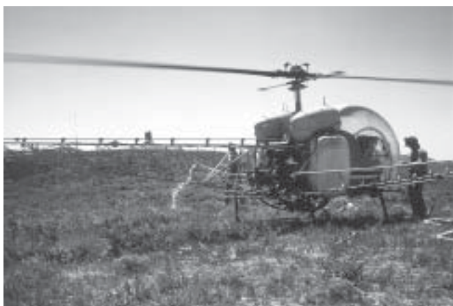
Figure 40 —Helicopter equipped with a boom sprayer.
