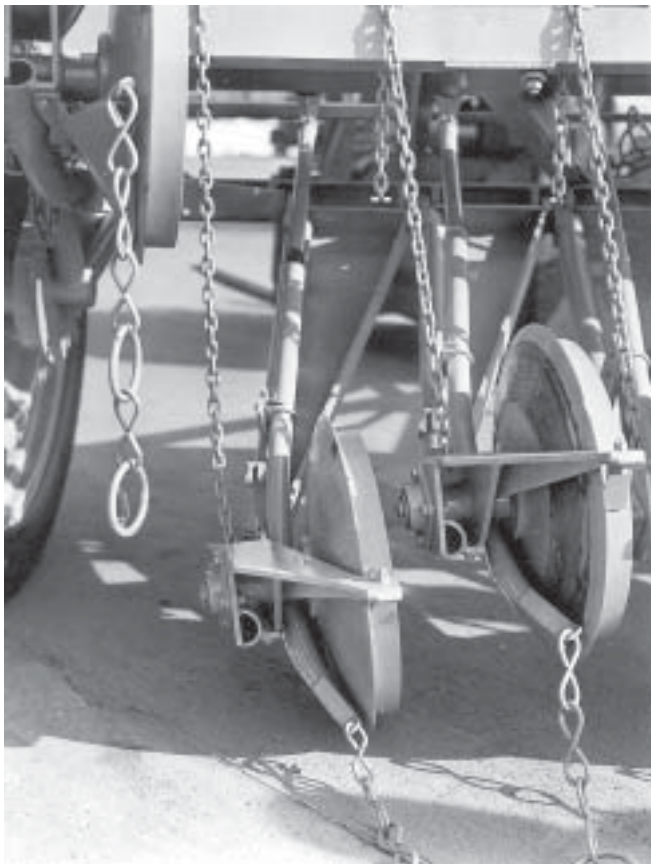
Figure 14 —Individually suspended arm on a Rangeland drill. Disk furrow openers are equipped with depth bands and a drag chain.
