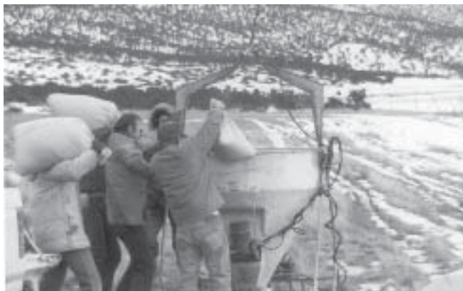
Figure 24 —Loading seed into a seed hopper suspended from a helicopter.
