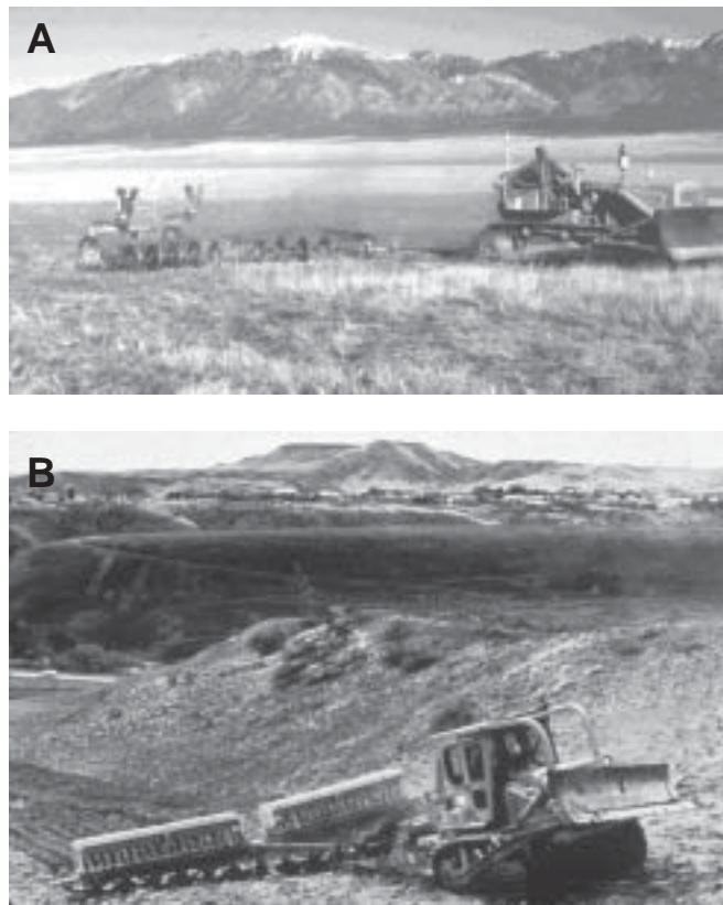
Figure 3 —Disk-chain. (A) Seed broadcast with electric powered cyclone seeder. (B) Disk-chain with seed boxes mounted above roller bar.
