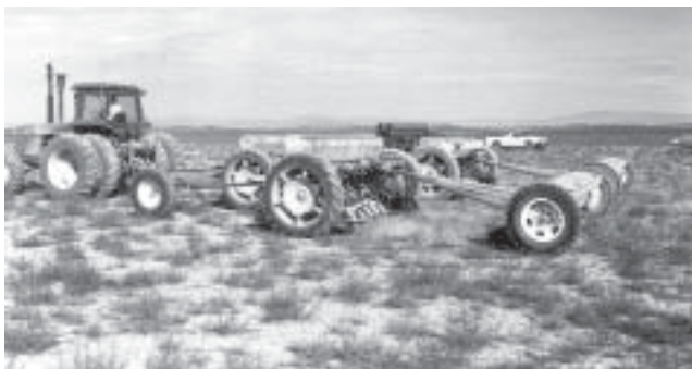
Figure 20 —Rangeland drills followed by sagebrush seeders and chain drags. Species requiring seed coverage are put through Rangeland drills. Species that require surface or near-surface seeding are run through the sagebrush seeders.
