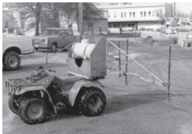
Figure 38 —Boom sprayer mounted on an all-terrain vehicle.
