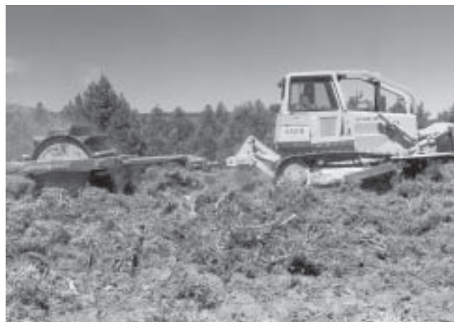
Figure 35 —Roller chopper being used to kill and cut up pinyon and juniper trees, create a seedbed, and cover seed.
