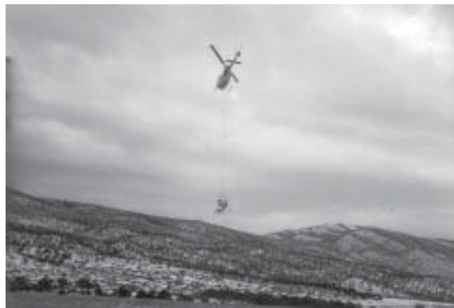
Figure 26 —Seeding small and irregular areas on rough terrain from a seed hopper suspended from a helicopter.
