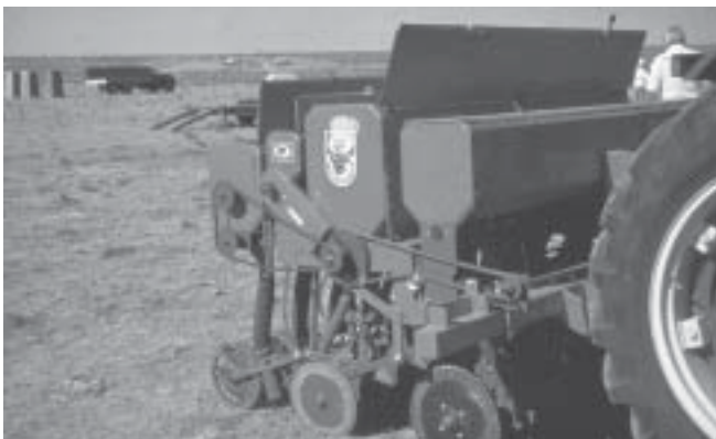
Figure 17 —Tye drill with four seed boxes and drops. Individual species or groups of species can be seeded at differing depths and rates and with or without press wheels.
