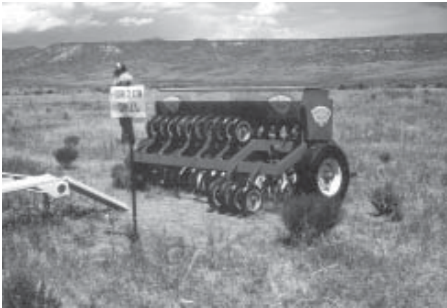
Figure 16 —Horizon drill with four press wheels down and 10 press wheels in the up position. Press wheels can aid in seedling establishment of some species. Species are separated in seed boxes according to seeding requirements.
