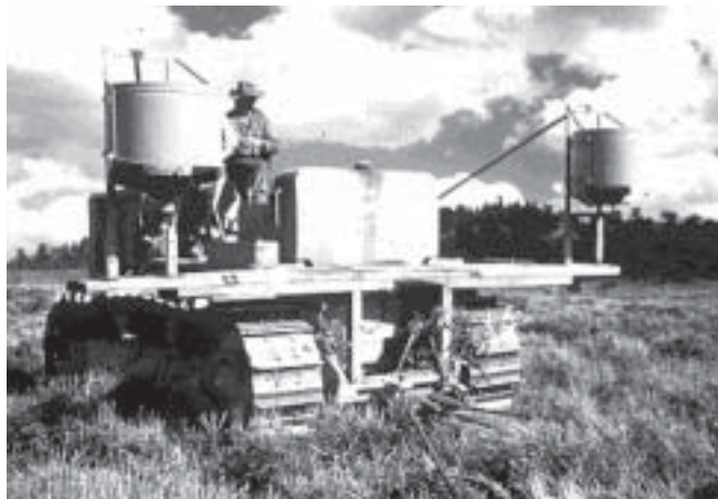
Figure 21 —Two electric broadcast seeders mounted on a crawler tractor that is pulling a pipe harrow.
