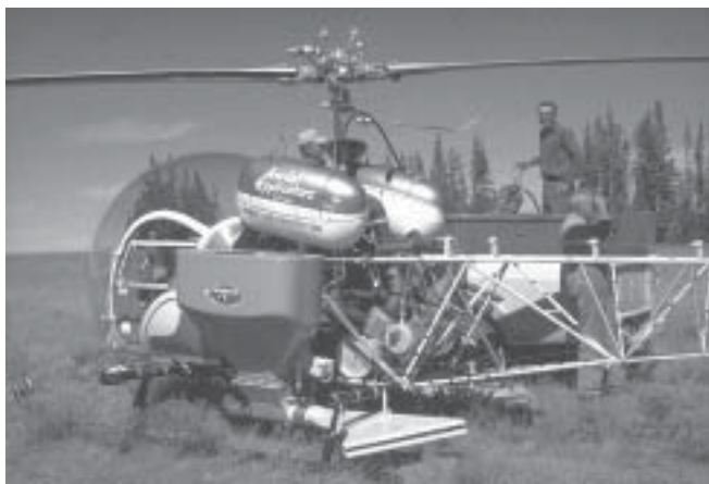
Figure 25 —Seed bins attached to a helicopter. Seed is dispersed by airflow.
