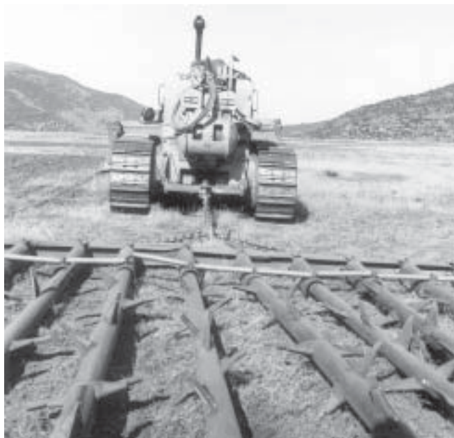
Figure 9 —Pipe harrow consisting of spreader-bar and trailing spiked pipes.
