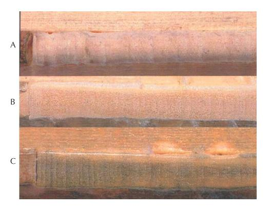
**Figure 1**—(A) Unsurfaced aspen core glued to wood mount, (B) surfaced and glued to wood mount, and (C) surfaced, stained, and glued to wood mount.
