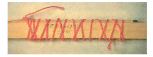
Figure 2—Aspen core glued and secured to wooden mount with string.
