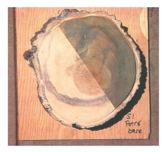
Figure 3—Surfaced aspen disk half stained and glued to wooden backing.
