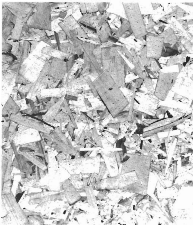
Figure 2.—Structural flakeboard manufactured from aspen.
