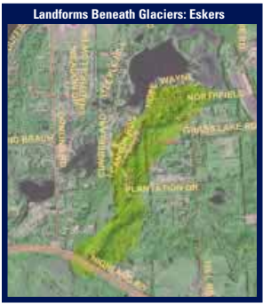
In some cases, long, winding rivers flow in tunnels beneath a glacier. Sediments deposited into these tunnels form ridges of layered sand and gravel that are left behind when the glacier recedes. These landforms are called eskers. The yellow highlighted portion in the aerial photograph above is an esker in Oakland County, Michigan.
