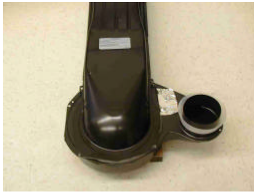
(a) Blower removed from the dryer
