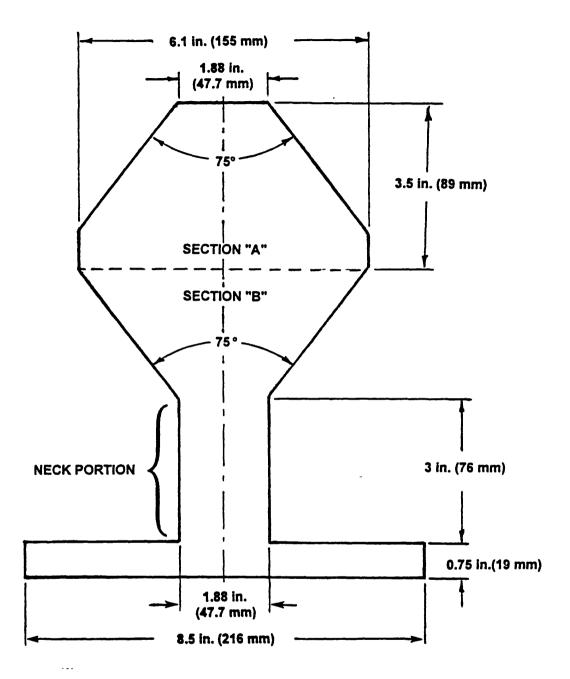
NOTE - Probe to be constructed from any rigid material 0.75 in. (19 mm) thick
