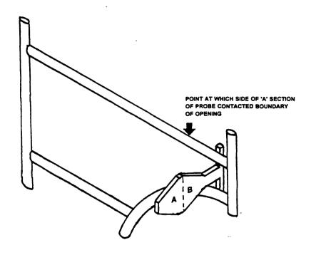
Fig 4 – Neck Portion of "B" Section of Probe Enters Completely into Opening
