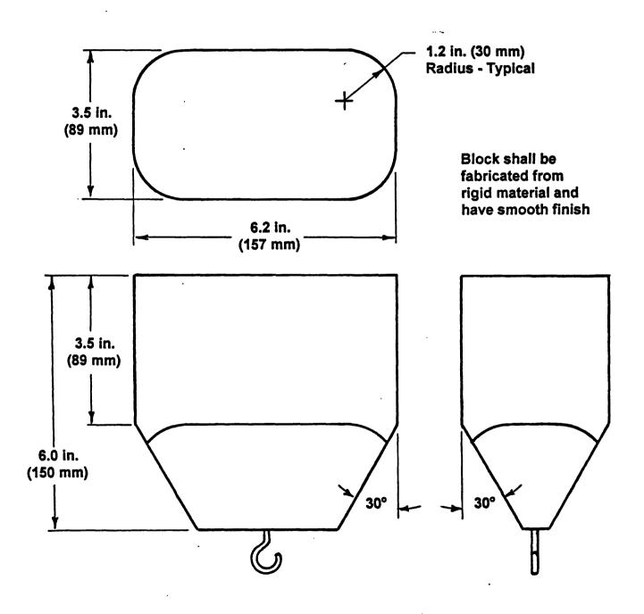
Figure 1 to Part 1213 - Wedge Block for Tests in § 1213.4(a), (b) and (c)
