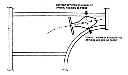
Fig. 3 – Motion of Test Probe Arrested by Simultaneous Contact With Both Sides of "A" Section of Probe and Boundaries of Opening
