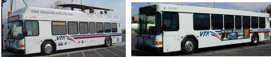
Figure 13. Fuel cell bus (left) and diesel bus (right)
