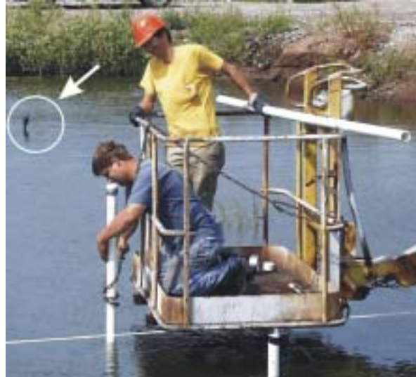
Technicians collect sediment core sample from ECGOx treatment area for PAH analysis. Note the ECGOx electrode (inside circled area).
