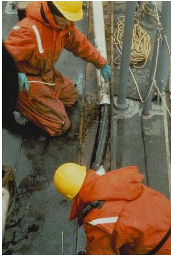
Scientists remove sediment core from vibracorer sampler's tube onboard the R/V Mudpuppy .
