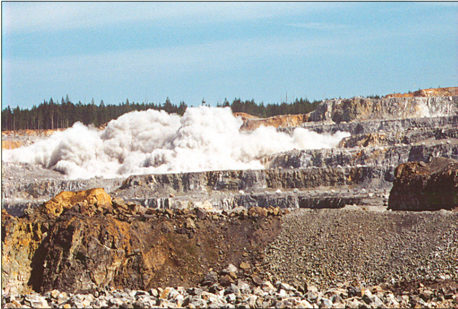
Figure 12. Rock is drilled and blasted for use as crushed stone. In some isolated areas where people are not located nearby, larger amounts of explosives may be used.
