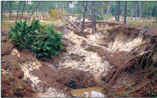
Figure 19. Human-induced sinkholes formed during the development of an irrigation well affected a 20-acre area and ranged in size from less than 1 foot to more than 150 feet in diameter. (Photograph courtesy Ann Tihansky, USGS.)
