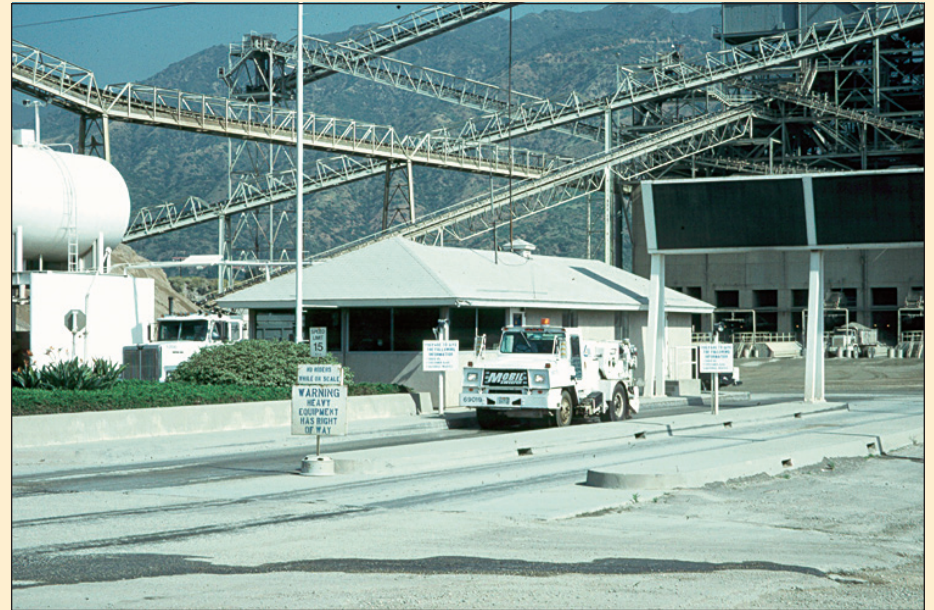
Figure 14. Dust control techniques include the use of water trucks and sweepers on haul.
