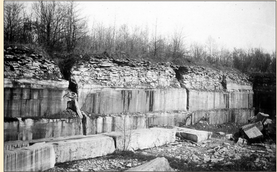
Figure 7. Working face of dimension stone limestone quarry in Lawrence County, Indiana, showing smooth surfaces from which large blocks have been removed. (USGS photographic library – Burchard #556.)
