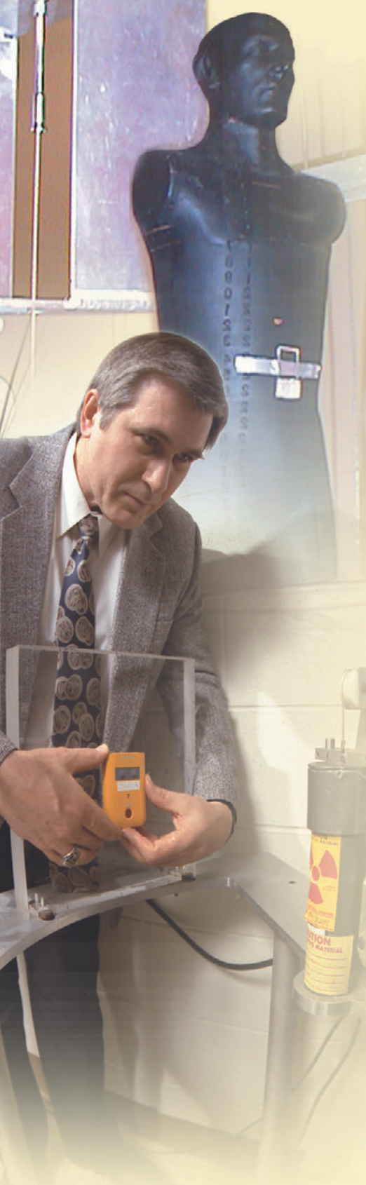
Using a phantom, Jim Bogard tests dosimeter responses to radiation from nearby sources.
