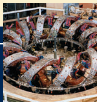
Advanced Toroidal Facility starts up for fusion energy research using a stellarator
