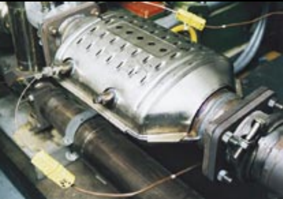
Prototype catalytic converter installed in engine test cell at Advanced Propulsion Tech Center. Digital image enhanced by Allison Baldwin.
