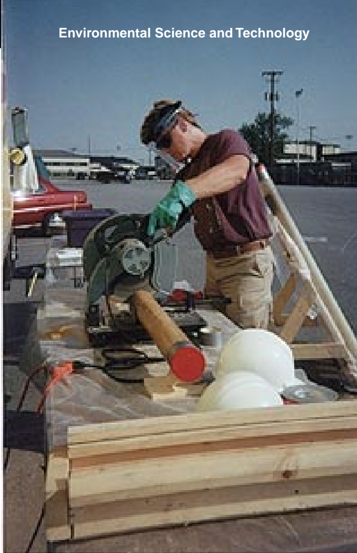
A member of the project team cuts a sediment core using sonic drilling at Dover Air Force Base. Photograph by Susan M. Pfiffner.
