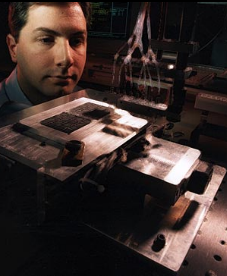
Mitch Doktycz checks the alignment of a robot's dispensing probes as he prepares to construct a set of flow-through genosensors. The dispensing probes transfer DNA sequences from microtiter plates to individual wells of the genosensors. Each genosensor measures less than half an inch on a side and contains almost 100 wells. A potential use of flow-through genosensors is rapid detection of genetic disease and other mutations. Photograph by Tom Cerniglio.
