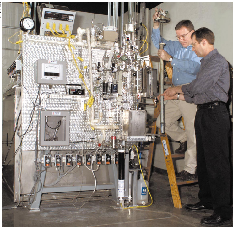
Jim Keiser and Mike Howell (on ladder) prepare to install samples in the Keiser Rig. This ORNL test furnace is used to expose samples of CFCC combustor liner materials and coatings to high-pressure water vapor similar to the combustion gases in gas turbines.
