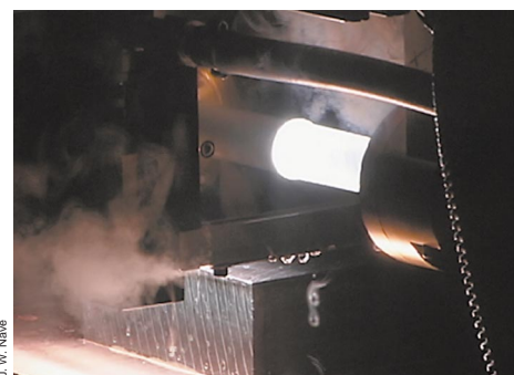
Views of the powerful plasma arc lamp at ORNL's Infrared Processing Center.
