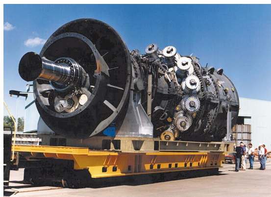
The new GE gas turbine produces power at 60% efficiency.
