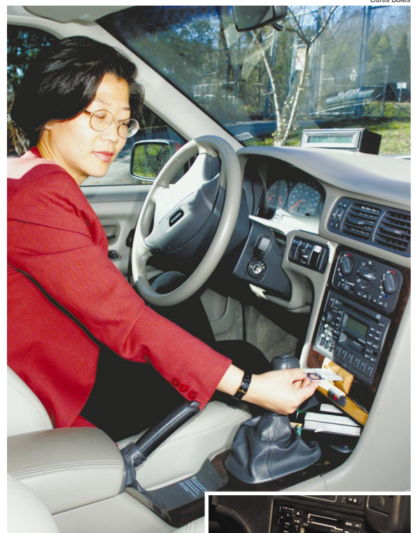
Pat Hu inserts her electronic driver's license in the Kittlelock smart ignition system inside the Volvo S-70 sedan. This car was driven at ORNL during a six-month field test in 1999.
