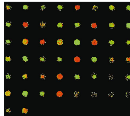
The red dots on the gene chip represent bacterial genes expressing themselves in the presence of oxygen. The green dots indicate bacterial genes expressing themselves when exposed to metal. The yellow dots denote genes expressed by bacteria under both sets of conditions.
