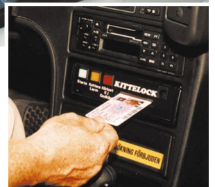
Pat Hu inserts her electronic driver's license in the Kittlelock smart ignition system inside the Volvo S-70 sedan. This car was driven at ORNL during a six-month field test in 1999.
