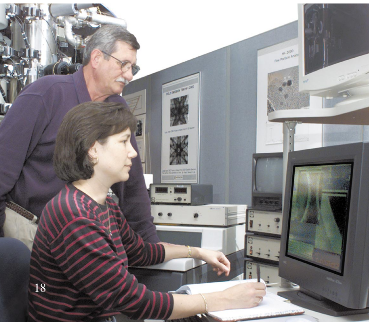
Karren More and Larry Walker use the Hitachi HF2000 transmission electron microscope to study fiber-matrix interfaces in continuous fiber-reinforced ceramic composites (CFCCs). These composites are similar to the CFCC combustor liners used in gas turbines for power production. More and Walker also use the JEOL 733 electron microprobe to analyze CFCCs after exposure to high-pressure water vapor in the ORNL test furnace and after actual engine tests.
