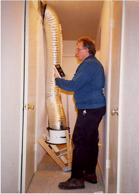
A duct blower is used by house inspectors and installation crews to identify and seal leaks in air distribution systems.
