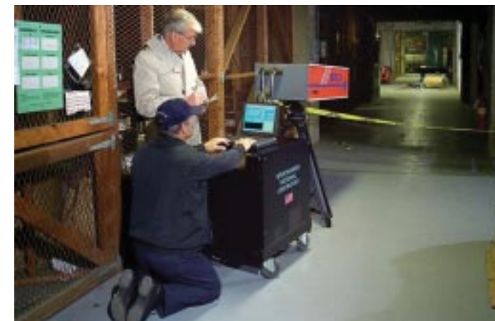
Brookhaven's one-of-a-kind chemical sensor — Mini-Raman LIDAR, or the Light Detection And Ranging device — is seen in action, surveying chemicals in a simulated event. The Mini-Raman LIDAR is a short-range, non-contact tool for identifying chemicals at a distance, without the need for collecting and handling a potentially hazardous or toxic sample.
