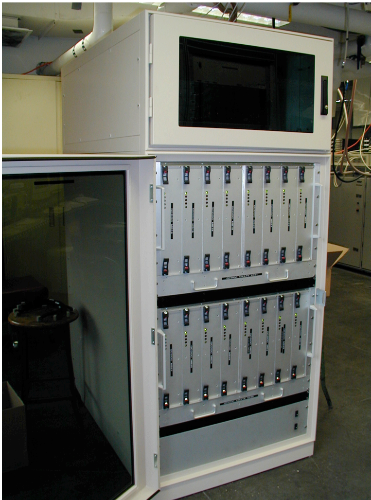
Figure 5: A QCDOC water-cooled rack which hold 1024 nodes on 16 motherboards mounted in two identical eight-motherboard crates.
