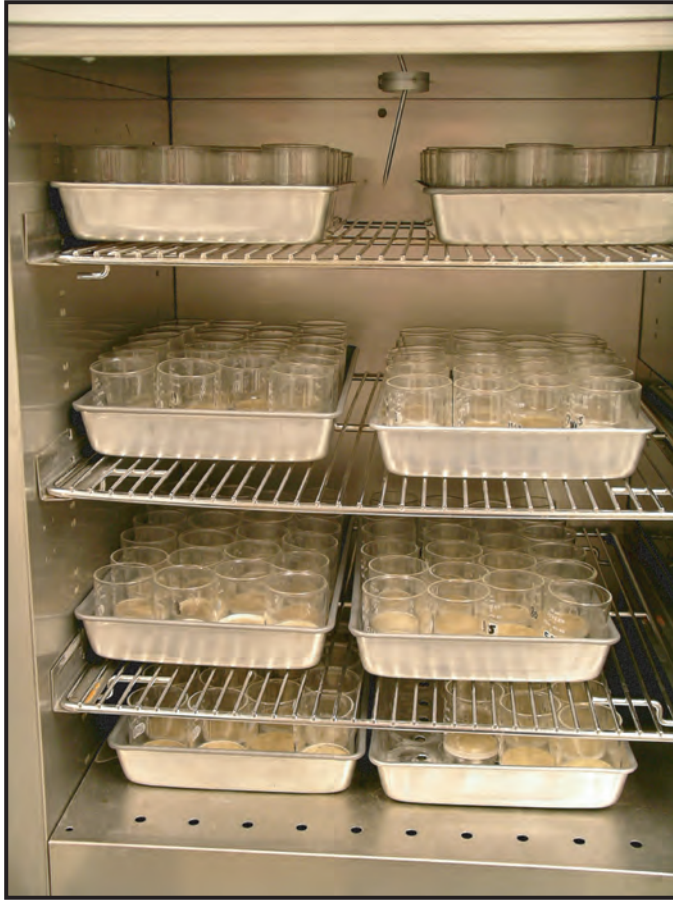
Figure 3. Convection oven for drying sediment in crucibles.
