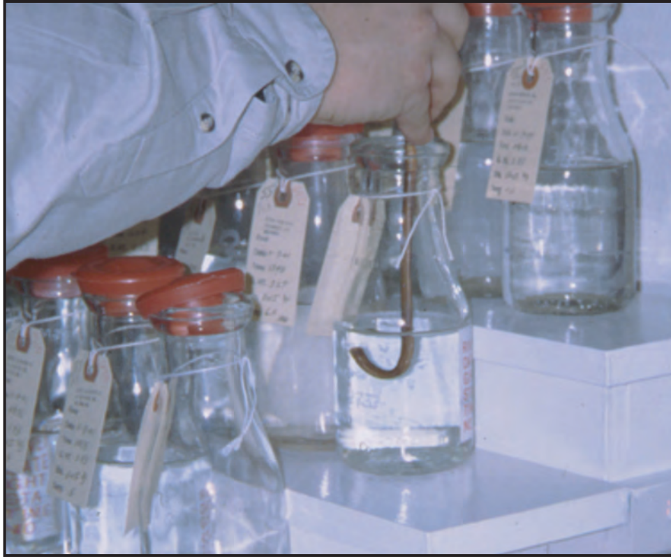
Figure 4. Vacuum-hose system and workbench for decanting water from suspended-sediment samples.
