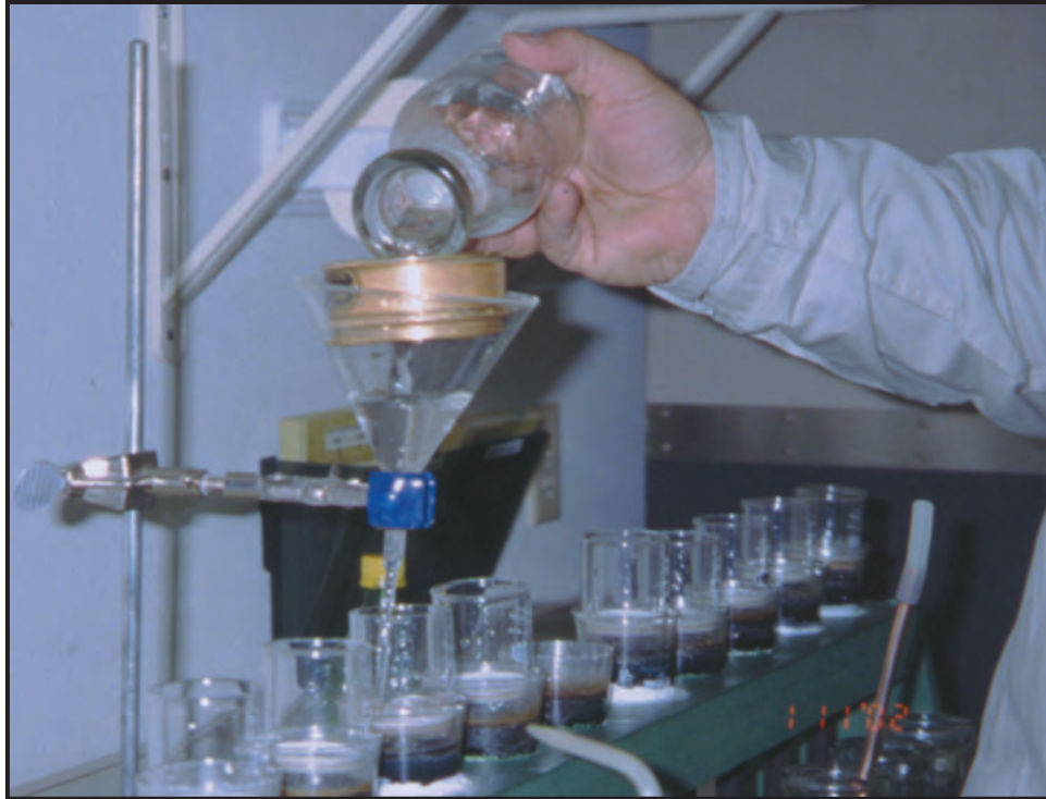
Figure 6. Suspended-sediment sample poured through a 0.062-millimeter sieve to separate sand from fine sediment.
