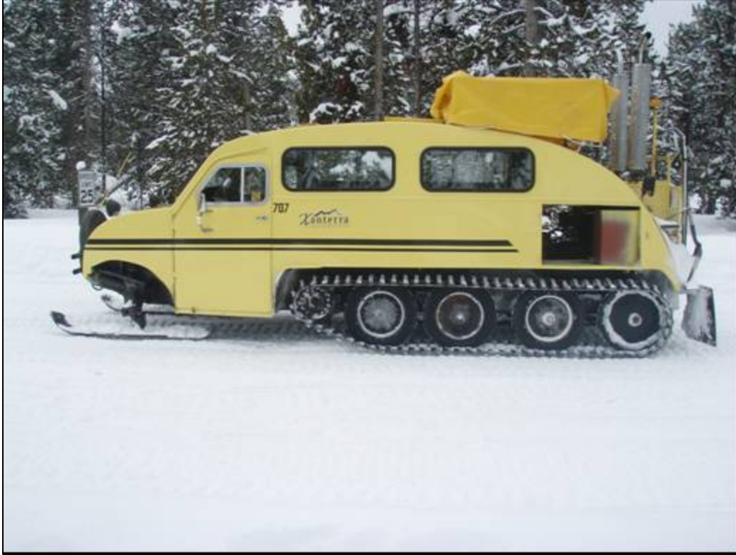
Figure 11. Purpose Built Bombardier B-12 with Skis and Tracks (Xanterra 707)
