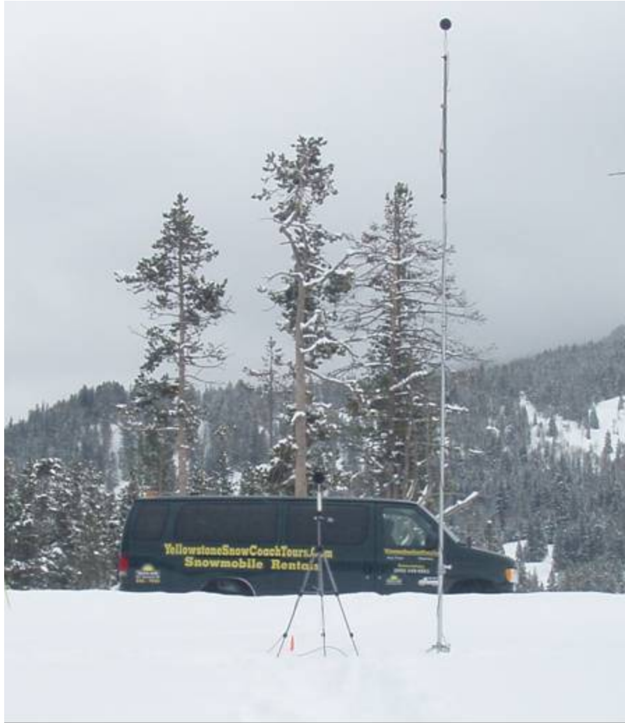
Figure 5. Measurement of Yellowstone Snow Coach Tours OSV Showing Line-of-Sight Blockage of Tracks due to Accumulated Snow
