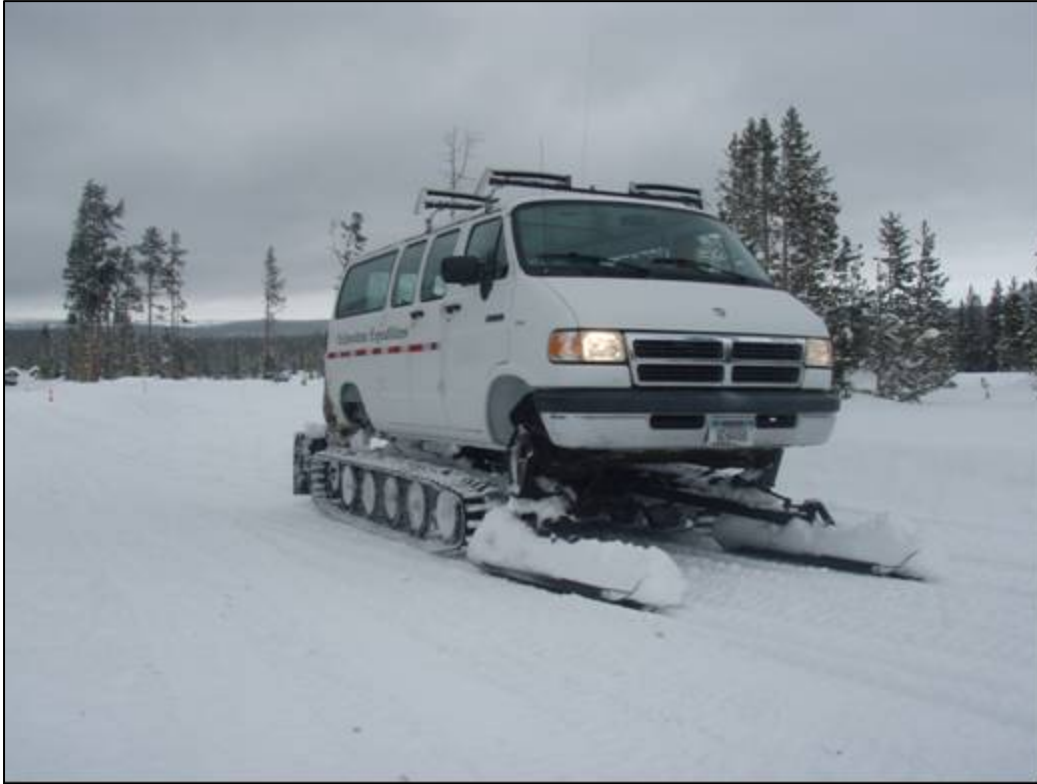
Figure 7. Customized Dodge B350 Van with “Snowbuster” Skis and Tracks (Yellowstone Expeditions)
