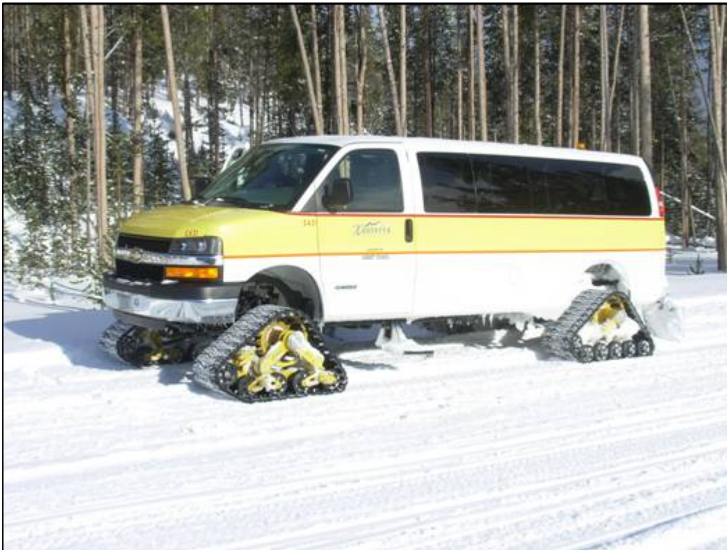
Figure 10. Customized Van with “Matracks” Tracks (Xanterra 431)
