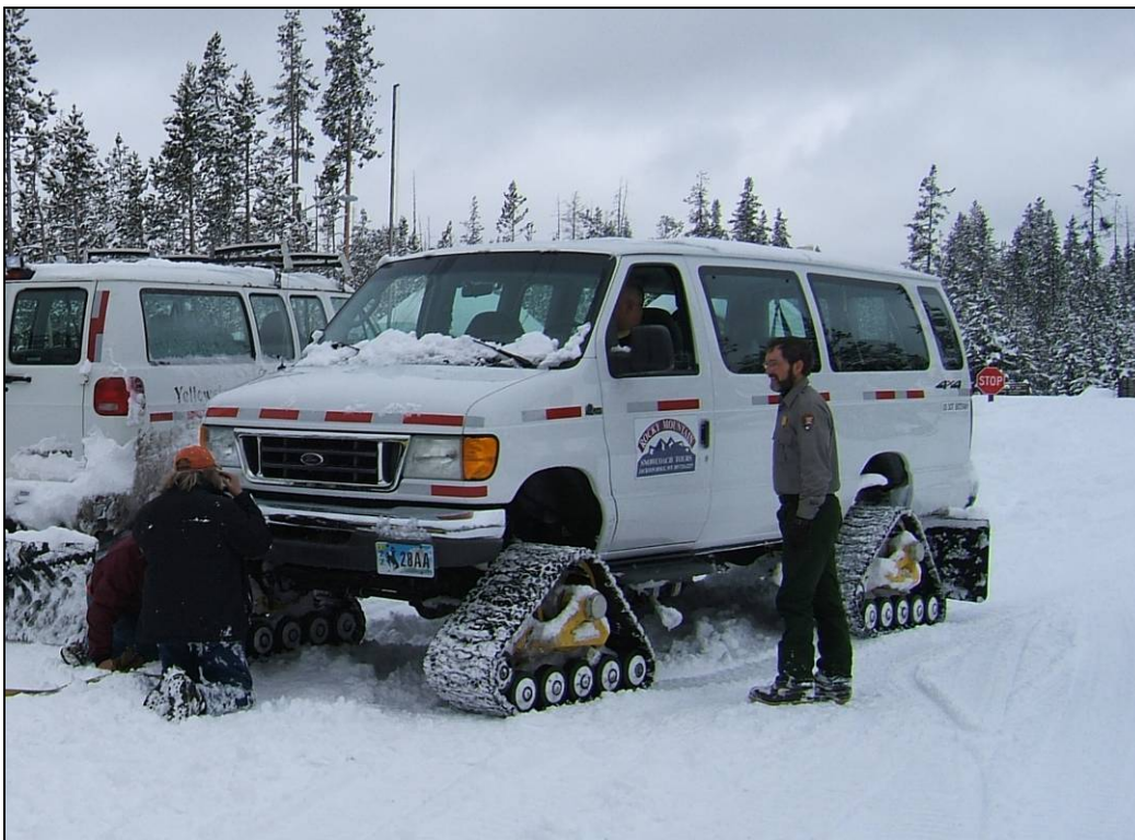
Figure 8. Customized Econoline 4 x 4 with “Mattracks” Tracks (Rocky Mountain SC Tours)
