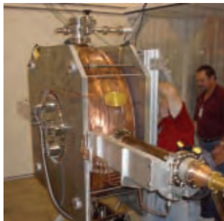
Muon Collider R&D RF cavity being prepared for tests at Fermilab.
