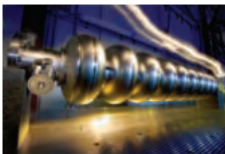
A superconducting ILC cavity Credit: Fermilab Visual Media Services
