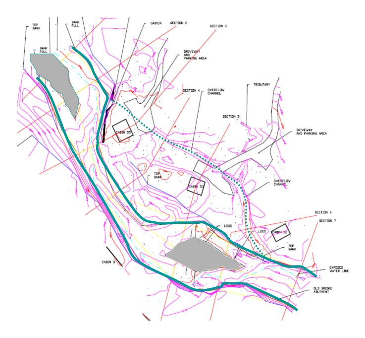
Figure 3. Plan view of area around Cabin 55. Current channel outline is a solid line. Side channel that would be re-opened is a dotted line. Cabins 55, 53, 52, are shown, and the streamside of cabin 3 is shown on the right bank. Downstream is to the right.
