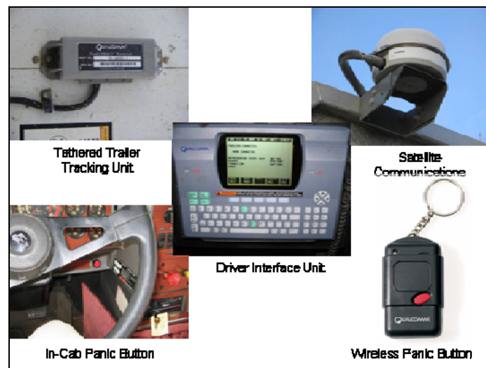
Figure 1. Technologies Installed for ESCT System Test
