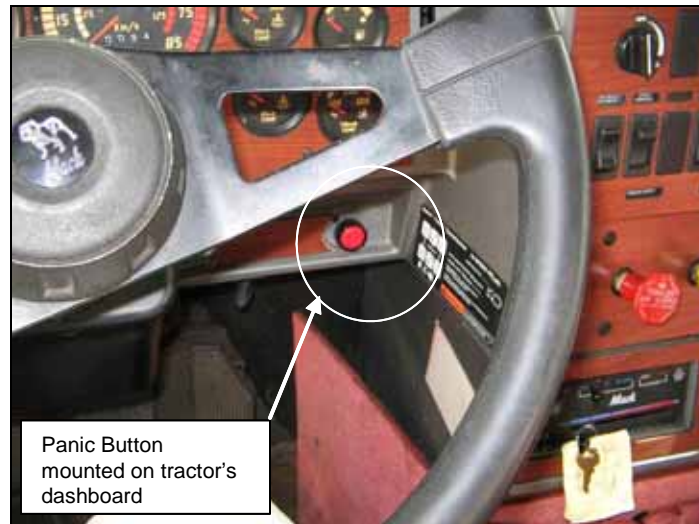
Figure 94. Wired Panic Button Installation in Shell Motiva Vehicle
