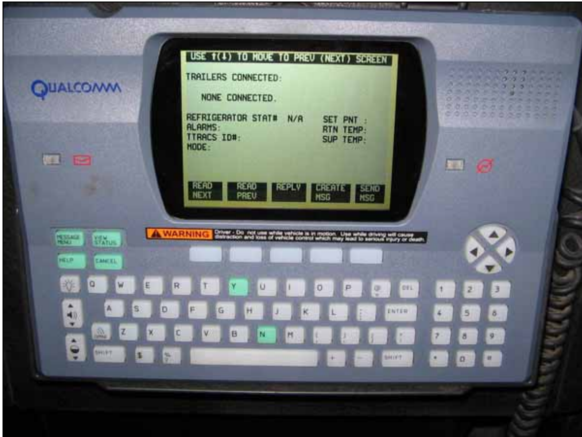
Figure 70. QUALCOMM Driver Interface Unit
